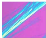
— PLM micrograph of NIST SRM 1866 chrysotile in 1.550 RI liquid, crossed with 550 nm retardation plate
