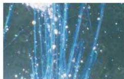
Figure D.4 — NIST SRM 1866 chrysotile in dispersion staining, viewed normal to polarizer vibration direction
