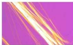
Figure D.2 — PLM micrograph of NIST SRM 1866 chrysotile in 1.550 RI liquid, crossed with 550 nm retardation plate
