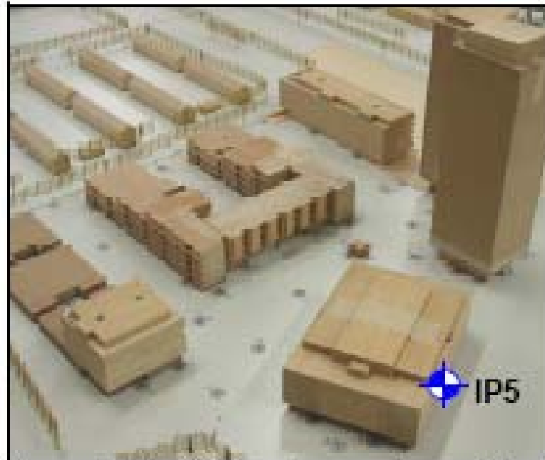
Figures 1+2: Inside view of the Peutz wind tunnel; detail of wooden scale model
