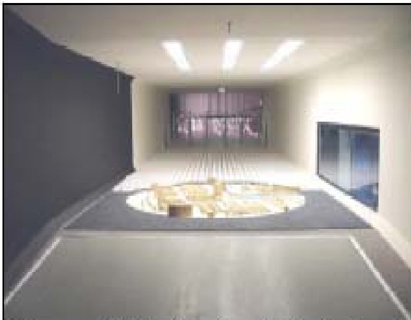
Figures 1+2: Inside view of the Peutz wind tunnel; detail of wooden scale model
