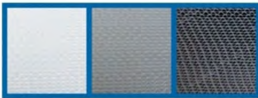
New and used filter (after 20.000 pages)
